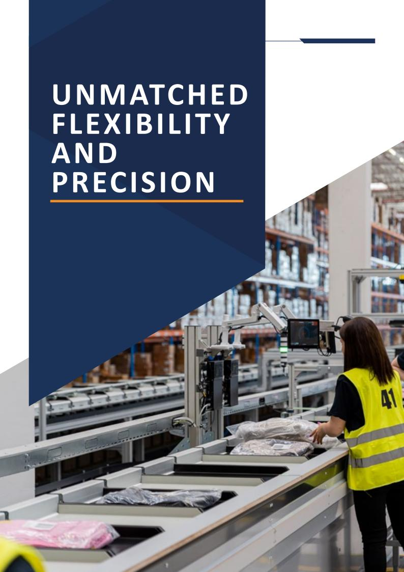
The EuroSort Push Tray Sorter is a reliable, high throughput single item sorting system. Suitable for flat, round, square, large, and small packages. The EuroSort Push Tray is a versatile sorter with a capacity of up to 24,420 uph, engineered for 24/7 use. Weight can go up to 20 kg per carrier, or 12 kg per tray. This sorter is the ideal system for any company that needs to handle high volumes of single items.
